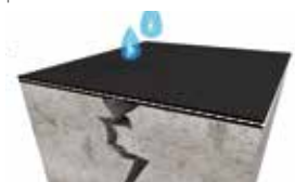
Crack bridging due to an embedded mesh. The mesh separates the top waterproofing layer from the crack and significantly helps to withstand permanent water pressure.
