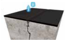
Crack bridging waterproofing: In this case due to elasticity and layer thickness. The waterproofing layer withstands permanent water pressure.
